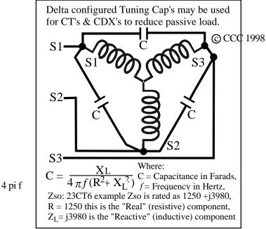
Fig. TC, Adding Tuning Capacitors for CT Type Loads
