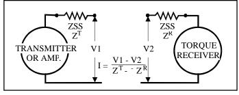
Fig. Vmm, voltage mismatch currents @ null
