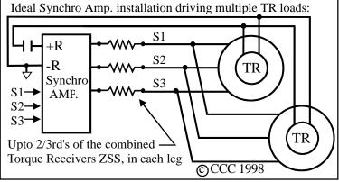
Load Balancing Resistors & Phase Shift added to Synchro Amp. The added resistors will effect the current flow through the synchro, the synchro signals however will still read 90 V.L-L. The higher the total line impedences, the lower the current flow at null.
