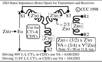
Fig. Zss, Driving Control Transformer (CT) and CDX Loads
