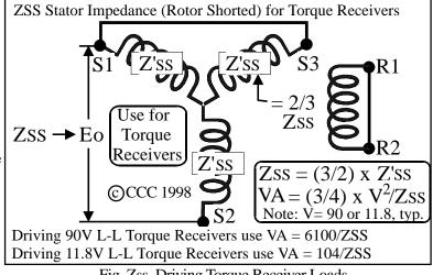
Fig. Zss, Driving Torque Receiver Loads
