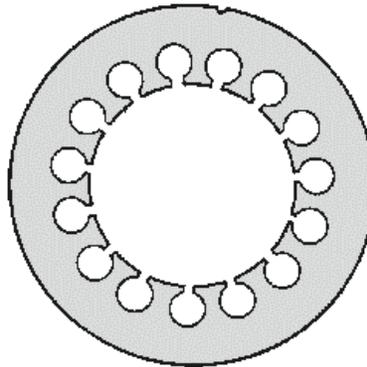
Figure 1-7B.—Stator lamination.
