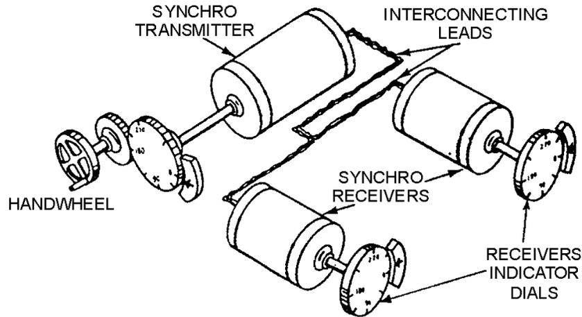
**TORQUE SYNCHRO SYSTEMS** are systems that use torque synchros to move light loads, such as dials and pointers.
