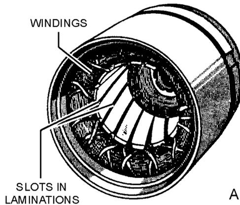
Figure 1-7A.—Typical stator.
