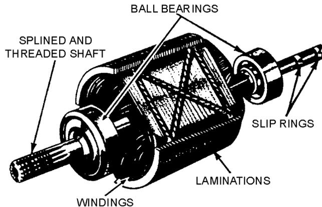
Figure 1-5.—Salient-pole rotor.
