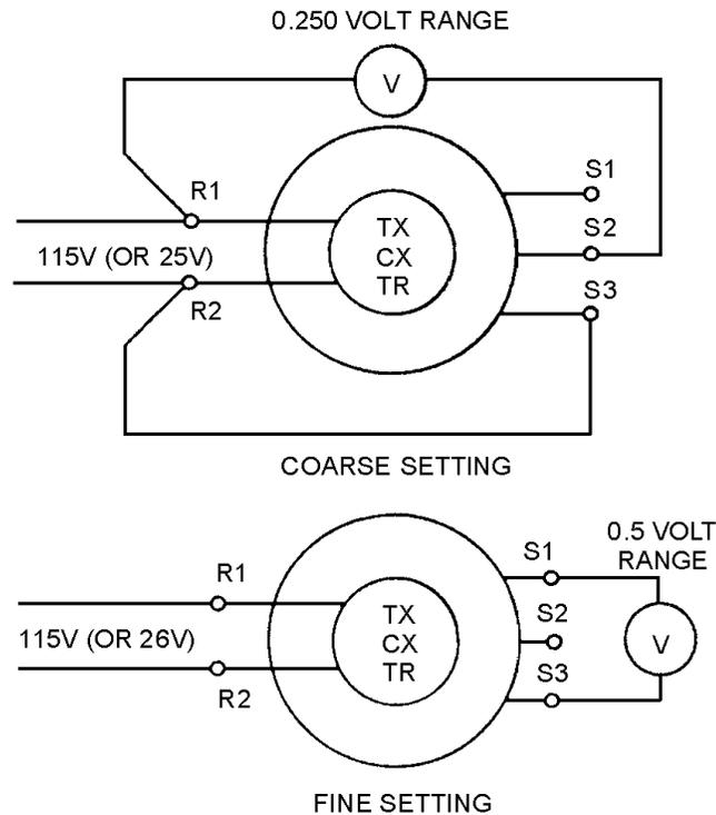
**ELECTRICAL-LOCK ZEROING METHOD** is perhaps the fastest. However, this method can be used only if the rotors of the synchros are free to turn and the leads are accessible. For this reason, this method is usually used on TRs.
