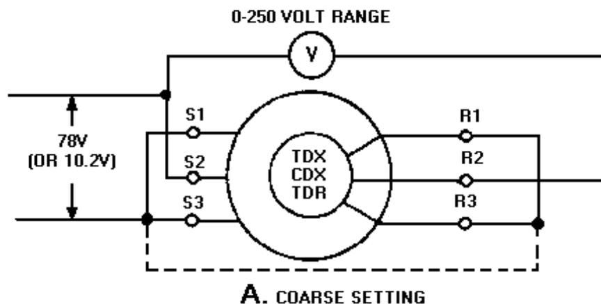
Figure 1-39A.—Zeroing differential synchros by the voltmeter method.
