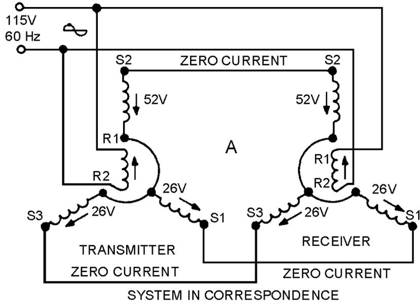
**SIGNAL** is defined as the angle through which a transmitter rotor is mechanically turned. This term has the same meaning as "transmitter's mechanical input."
