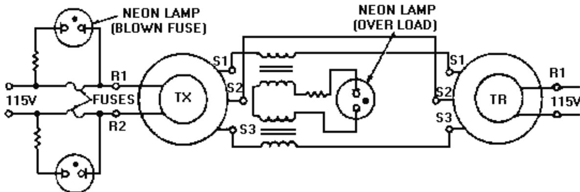
**SYNCHRO TROUBLESHOOTING** is the locating or diagnosing of synchro malfunctions or breakdown by means of systematic checking or analysis. This is done by using trouble indicators, trouble tables furnished by manufacturers, known operating voltages as references, and synchro testers.
