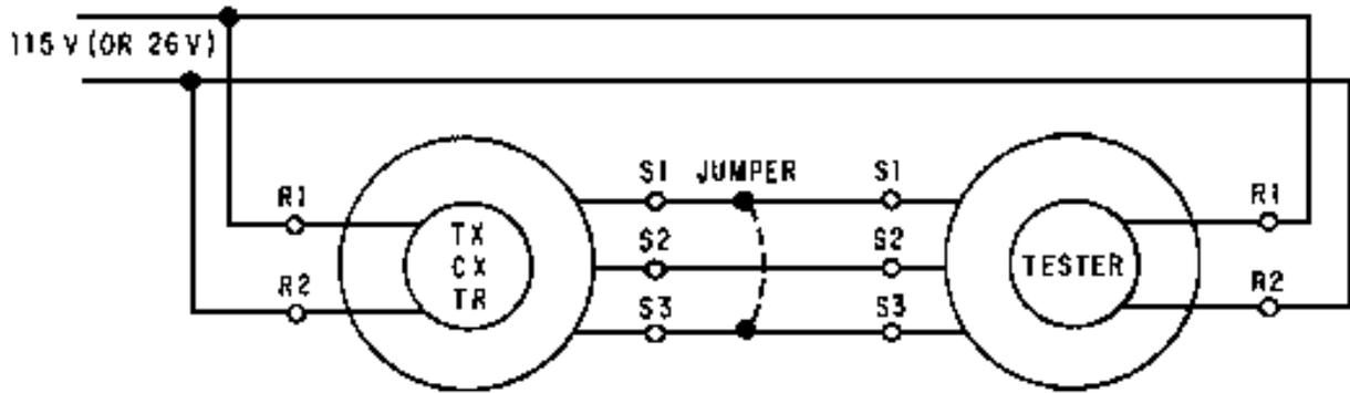
Figure 1-43.—Zeroing a synchro using a synchro tester.
