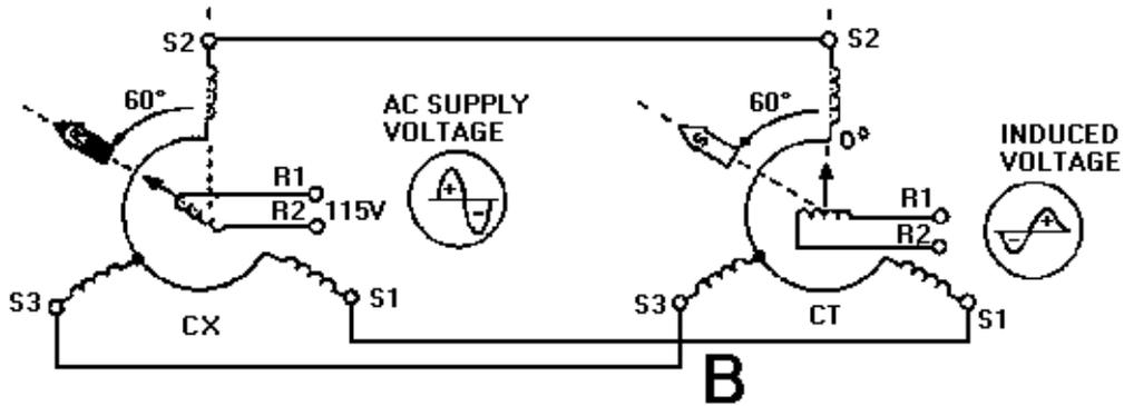
Figure 1-27B.—Control synchro system operation.
