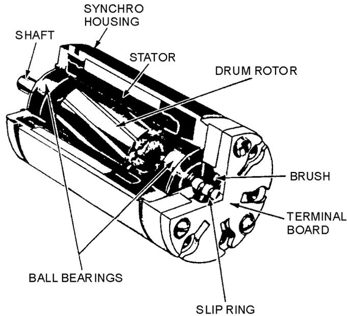
A **SYNCHRO ROTOR** is composed of either a single coil of wire wound on a laminated core or a group of coils wound in slots in a laminated core. The laminated core is rigidly mounted on a shaft that is free to turn inside the stator. Two slip rings are mounted on one end of the shaft to supply excitation voltage to the rotor. There are two common types of synchro rotors - the salient-pole rotor and the drum or wound rotor.
