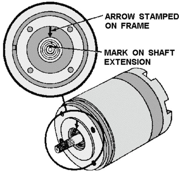
Figure 1-37.—Coarse electrical zero markings.
