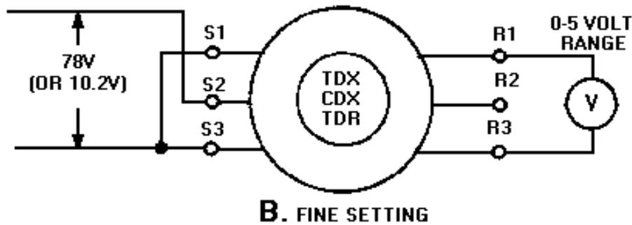
Figure 1-39B.—Zeroing differential synchros by the voltmeter method.
