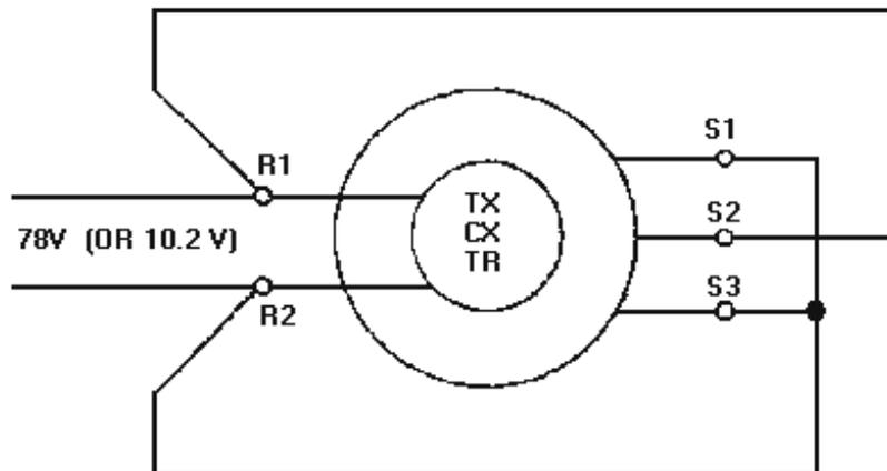
The **SYNCHRO-TESTER ZEROING METHOD** is potentially less accurate than the voltmeter or electric lock methods. This is because the dial on the tester is difficult to read and may slip from its locked position.
