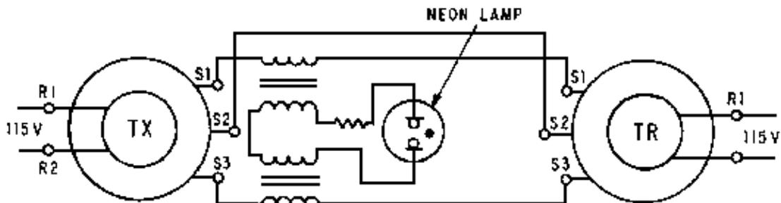
Figure 1-44.—Overload stator current indicator.
