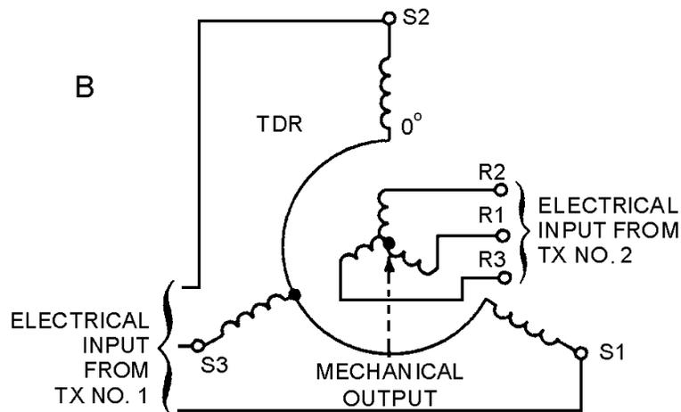
The **TX-TDX-TR SYSTEM** performs subtraction when the system contains standard synchro connections. Addition can also be performed with this system by reversing the S1 and S3 leads between the TX and the TDX, and the R1 and R3 leads between the TDX and the TR. Remember, this system works like a basic synchro system when the rotor of the TDX is on 0°; in this condition the TR rotor follows the TX rotor exactly.
