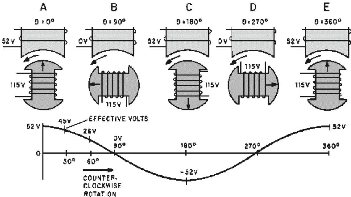
The **SYNCHRO RECEIVER (TR)** is electrically identical to the synchro transmitter. The receiver, however, uses some form of rotor damping that is not present in the transmitter. This real difference between a synchro transmitter and a synchro receiver lies in their applications. The receiver converts the electrical data, supplied to its stator from the transmitter, back to a mechanical angular output through the movement of its rotor.
