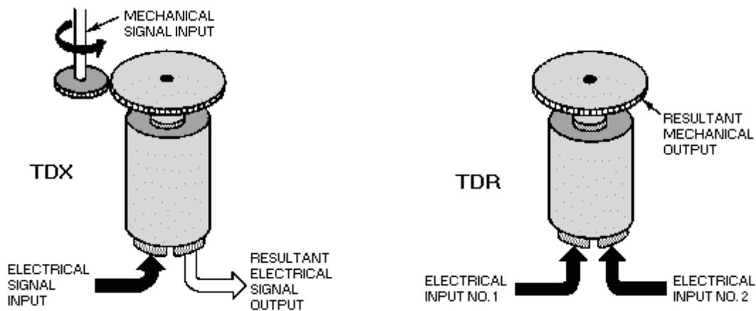
Figure 1-18.—Torque differentials.
