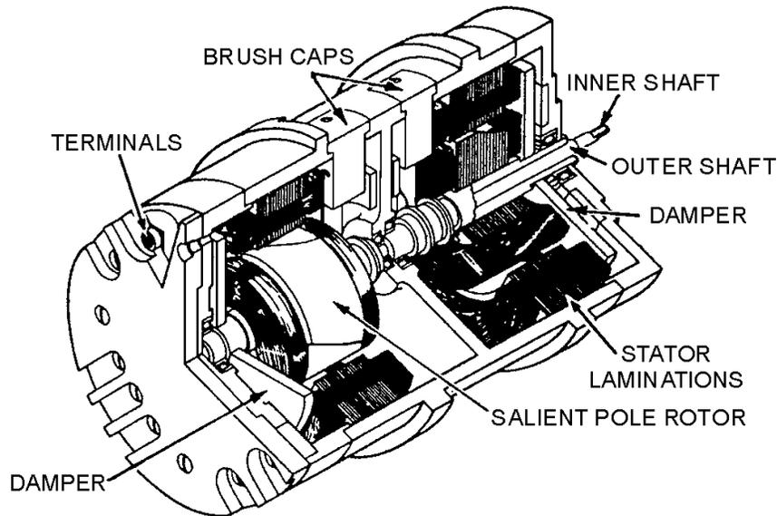
Figure 1-35.—Cutaway view of a double receiver.
