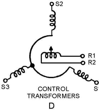
Figure 1-3D.—Schematic symbols for synchros.
