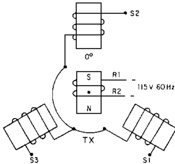
The **SYNCHRO TRANSMITTER (TX)** converts a mechanical input, which is the angular position of the rotor, into an electrical output signal. The output is taken from the stator windings and is used by a TDX, a TDR, or a TR to move light loads, such as dials and pointers.
