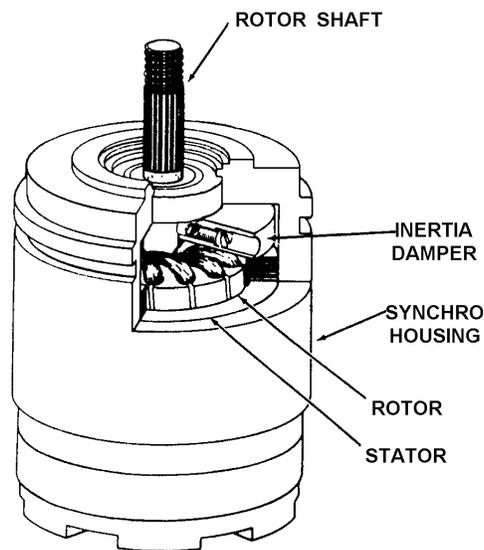
A **TORQUE SYNCHRO SYSTEM** consists of a torque transmitter (TX) electrically connected to a torque receiver (TR). In this system, the mechanical input to the TX is transmitted electrically to the TR. The TR reproduces the signal from the TX and positions either a dial or a pointer to indicate the transmitted information.
