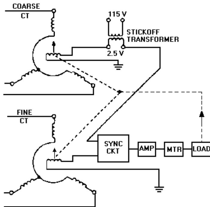
**ELECTRICAL ZERO** is the reference point for alignment of all synchro units.
