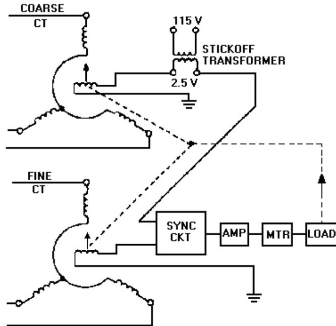
Figure 1-36.—Dual-speed synchro system using a stickoff transformer.
