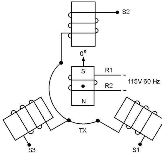
Figure 1-13.—Synchro transmitter.
