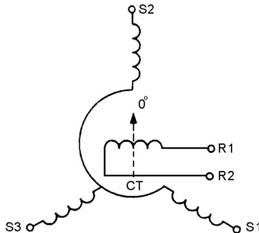
**ERROR SIGNAL** is the name given to the electrical output of a CT. The reason is that the electrical output voltage represents the amount and direction that the CX and CT rotors are out of correspondence. It is this error signal that eventually is used in moving the load in a typical servo system.
