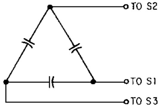
Figure 1-29.—The synchro capacitor.
