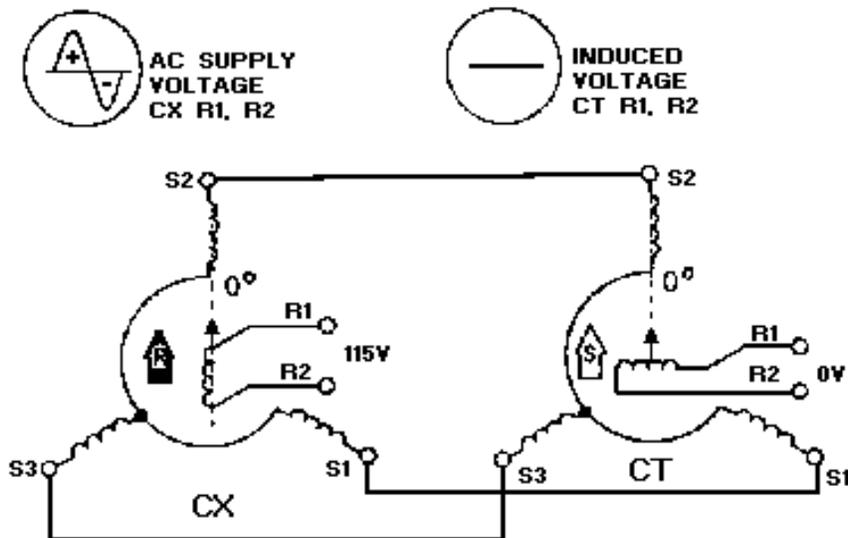
Figure 1-25.—CX-CT system operation with rotor in correspondence.
