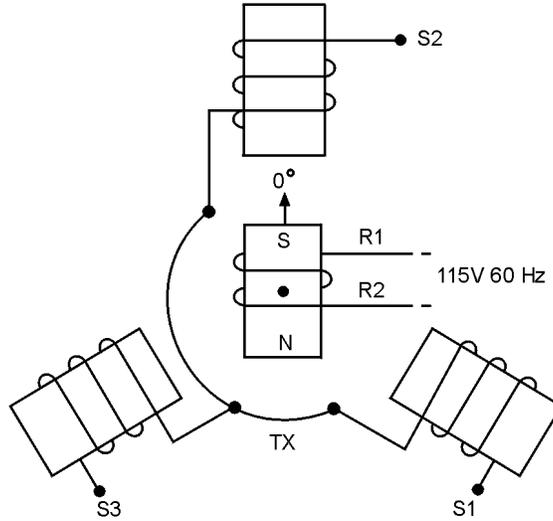
Figure 1-13.—Synchro transmitter.
