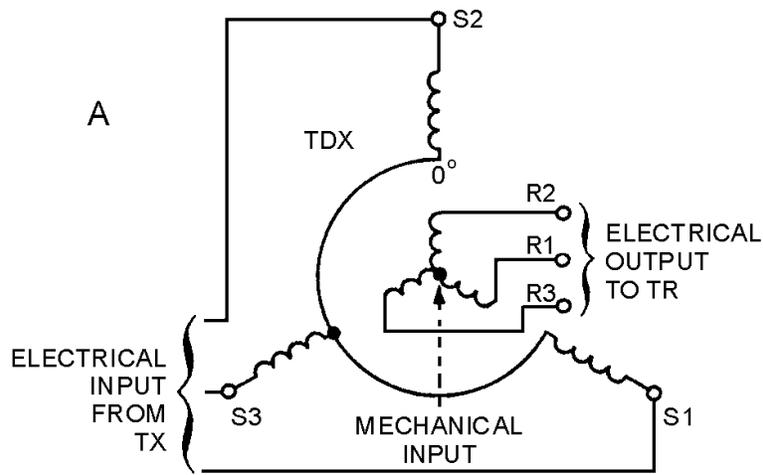
The **TORQUE DIFFERENTIAL RECEIVER (TDR)** is electrically identical to the TDX. The only difference in their construction is that the TDR has some form of damping. The real difference between the two differentials lies in their applications. The TDR has two electrical inputs, one to the rotor and the other to the stator. The output is the mechanical position of the rotor. As is the case with the TDX, the addition or subtraction function of the TDR depends upon how it is connected in the system.
