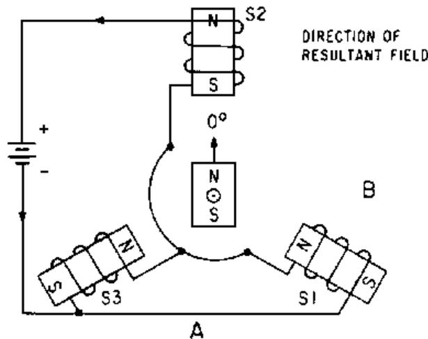
Figure 1-9.—Operation of three electromagnets spaced  $120^\circ$  apart.
